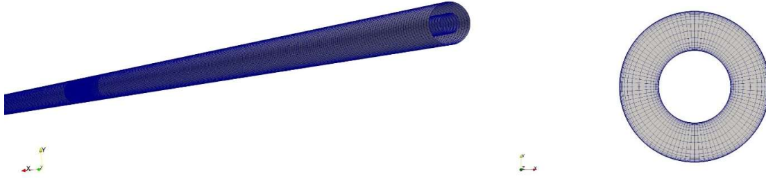
Figure 31: (left) Axial view of the structured hexahedral mesh used in the cantilevered-rod case. (right) Cross-section of the annular computational grid.
