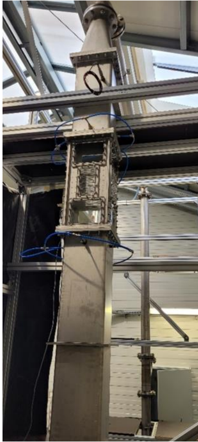
Figure 3: Test section with inlet and outlet channels
