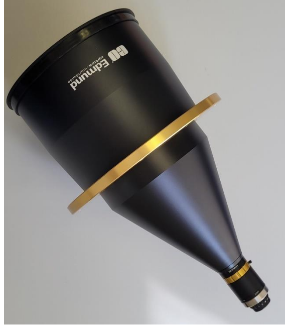
Figure 17: Telecentric lens for PIV measurement
